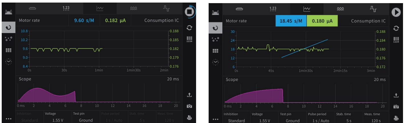
Figure 35: Left: good watch without chopping pulse. Right: Bad watch without chopping pulse.
