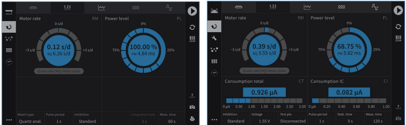
Figure 32: Measurement of motor rate deviation (RM), quartz rate deviation (RQ), power level (PL) and pulse duration (PW) Left: With QuartzSensor/terminal via an inductive/capacitive sensor. Right: With QuartzMaster@ /Terminal via the current measurement.
