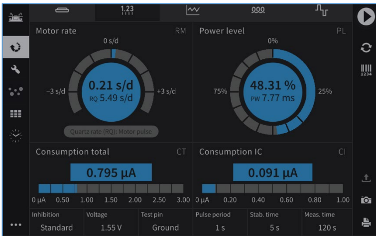
Figure 31: Current consumption of a quartz watch. Total current (CT) and IC current (CI)
