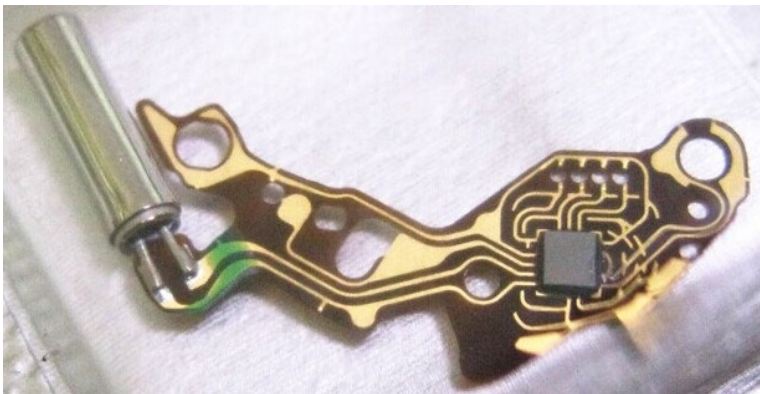
Figure 26: Image of the circuit board with watch IC and adjustment by connecting integrated fixed capacitors via solder bridges.
