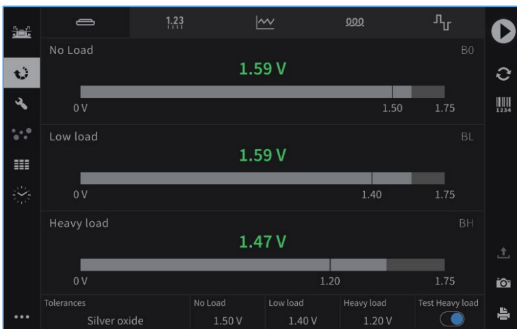
Figure 30: Battery voltage measurement without load, with low load and high load.
