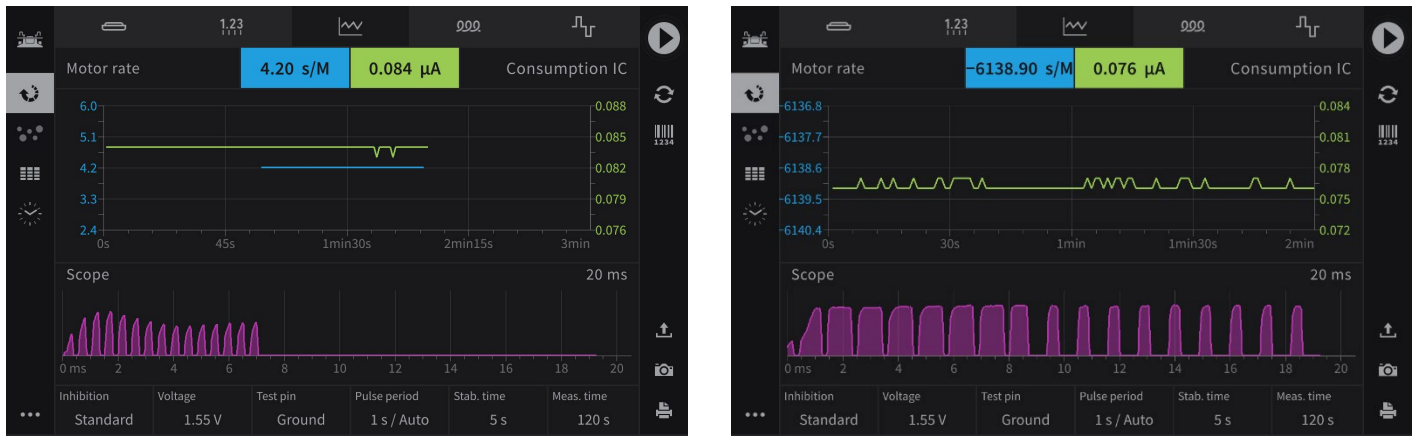
Figure 34: Left: good watch with chopping pulses. Right: bad watch with chopping pulses.
