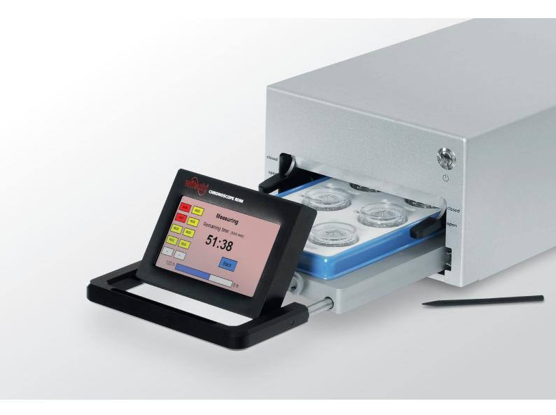
The Chronoscope RDM (Réserve de Marche) measures the power reserve of mechanical watch movements or watches in a simple and time-saving way. The power reserve measurement is accurate to the minute and takes place autonomously, so that the process can be carried out regardless of the time of day or even over the weekend.
